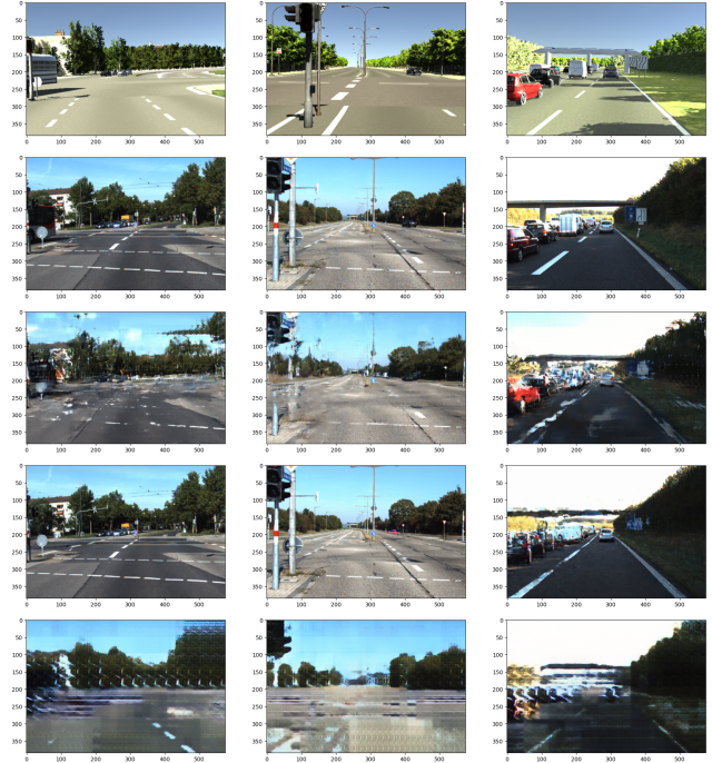
Figure 6. Input synthetic images and their corresponding Ground Truth and Generated images. Row 1: Input Image, Row 2: Ground Truth Row 3: U-Net, Row 4: ViT and Row 5: Swin
